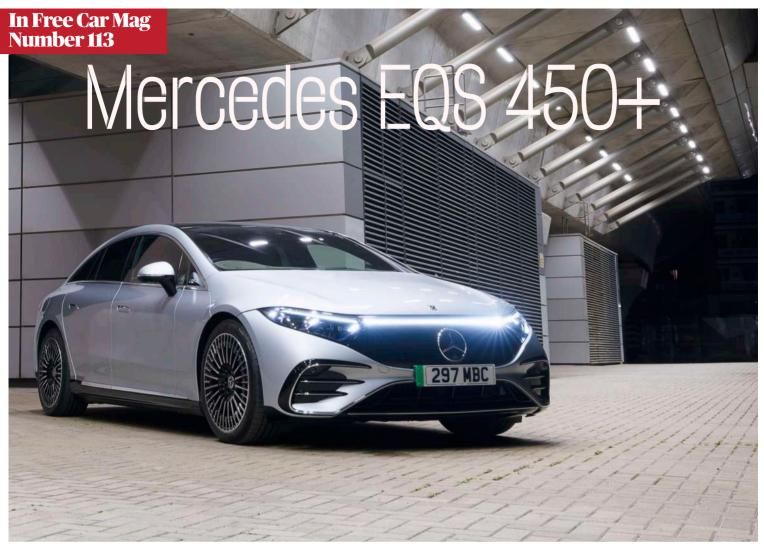
he Mercedes EQS is the S-Class of Electric Cars. It was the first EQ model based on the MEA EV platform and is powered by a water-cooled motor sending torque to the rear wheels through a single-speed gearbox. Prices start from around £100,000 for the EQS 450+ AMG Line, but add in another £7k for this 450+ Luxury. In fact, Mercedes seems to like its £7k plus increments. It produces about 333bhp and 568Nm of torque
