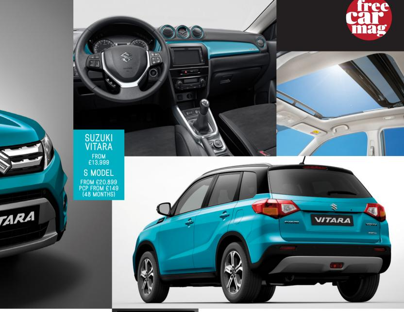
When the sunroof is closed, the glass panels have a combined length of 1,000mm. When the sunroof is open, the opening has a length of 560mm (one of the largest in its class), giving everyone inside an invigorating openroof experience.
